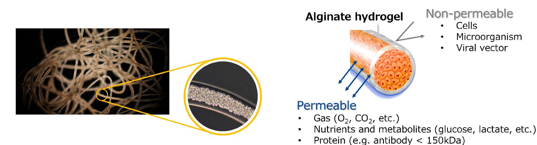
Figure 1. CellFiber ® cell encapsulation technology
